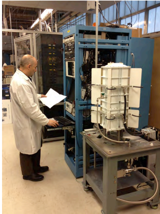
FIGURE 3-7 | ASRG ENGINEERING UNIT 2
