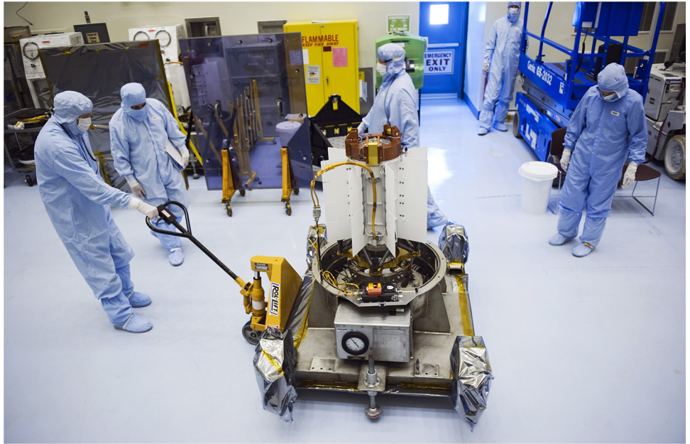
Figure 3: Multi-Mission Radioisotope Thermoelectric Generator (MMRTG) for the Curiosity Rover at Kennedy Space Center
