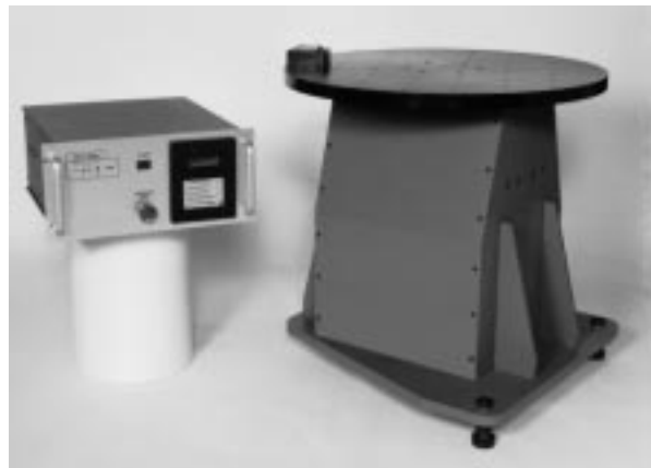
Figure 9-22: A typical rate table used for tuning gyros.
