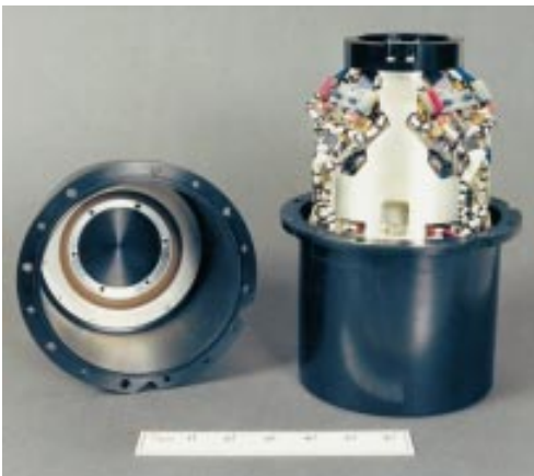
Figure 9-17: A strapdown IMU containing three accelerometers and three ring laser gyros.
