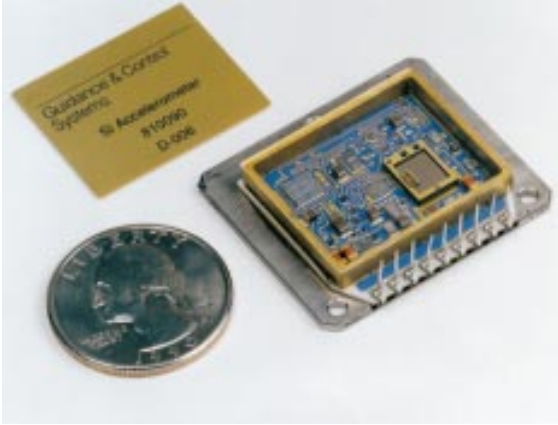
Figure 9-13: An integrated circuit accelerometer rated at over 100 g.
