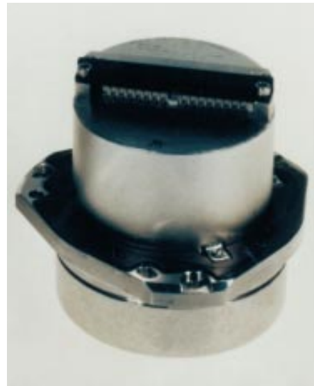
Figure 9-7: A DTG dynamically tuned spinning mass gyro.
