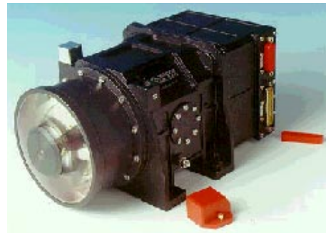
Figure 9-3: A high resolution gyro-astro compass.
