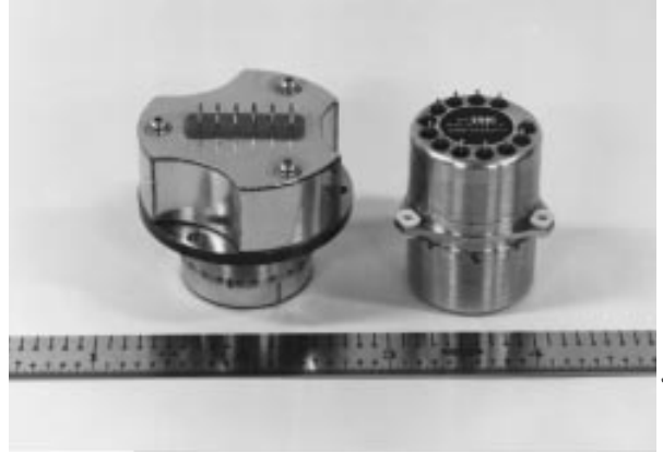
Figure 9-5: Two force rebalance accelerometers that can be built with any of a wide range of performance capabilities.
