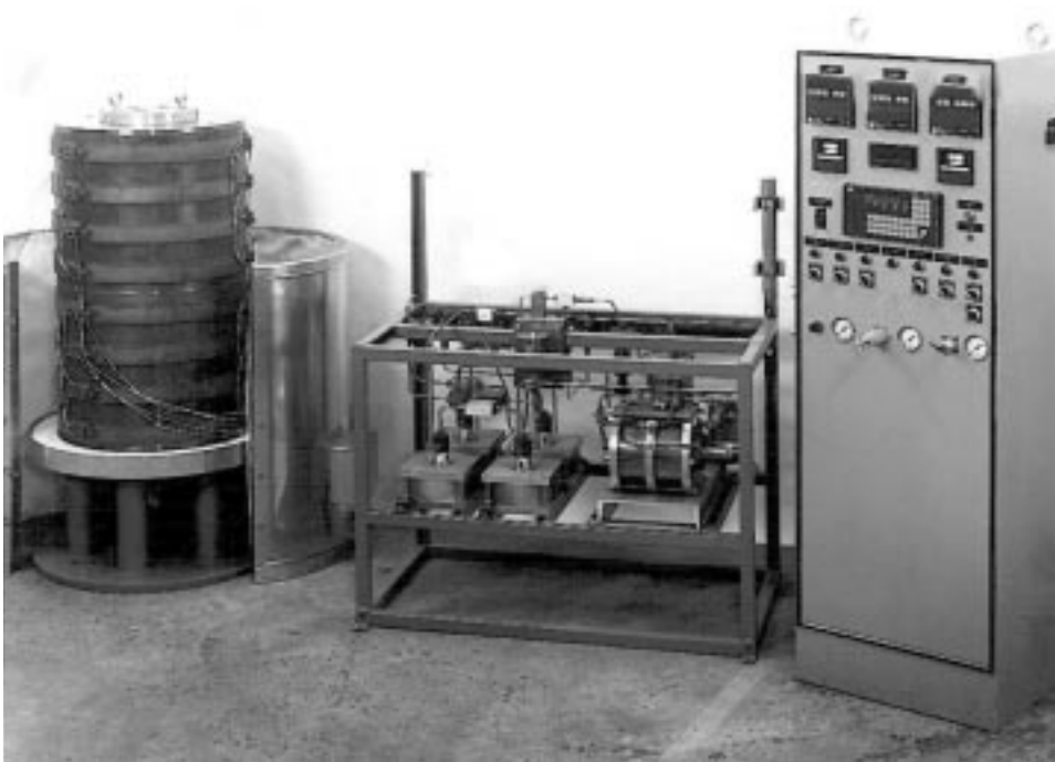
Figure 7-1: A laboratory-sized isostatic press showing its three main components: pressure chamber, pressure generator, and control console.
