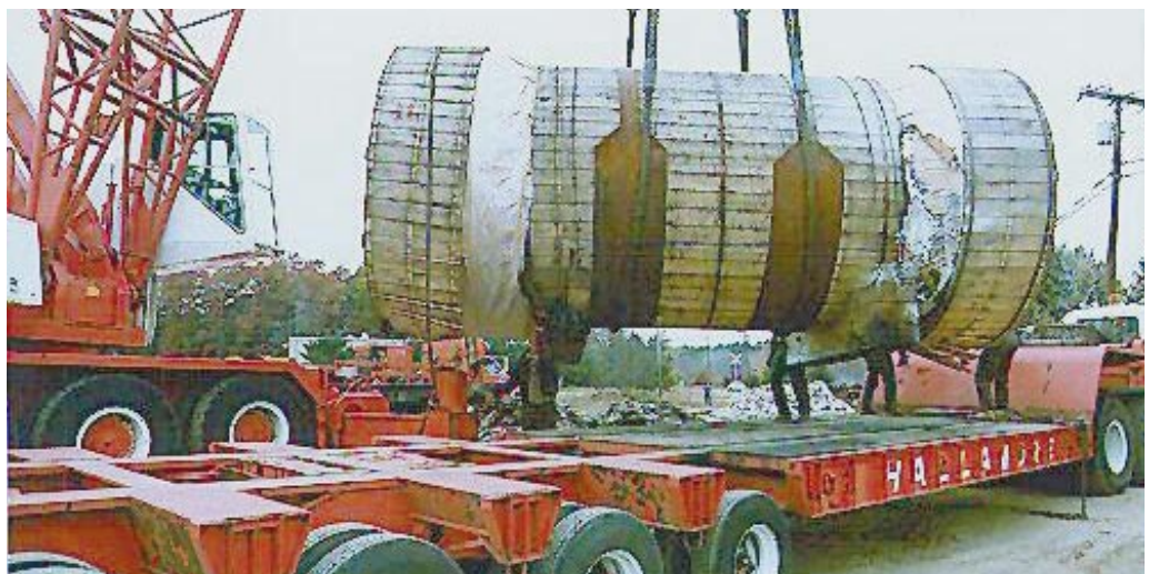
Figure 7-7: Alternative shipping crate for an isostatic press.
