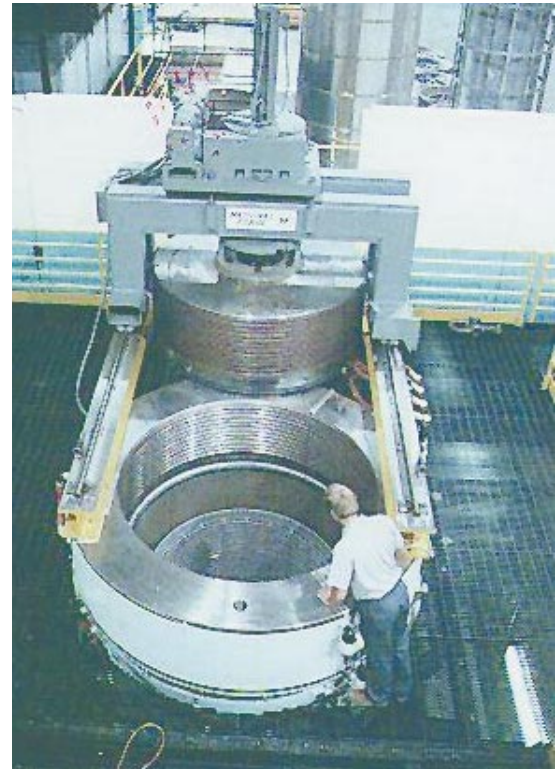
Figure 7-3: A very large isostatic pressure vessel and threaded plug.
