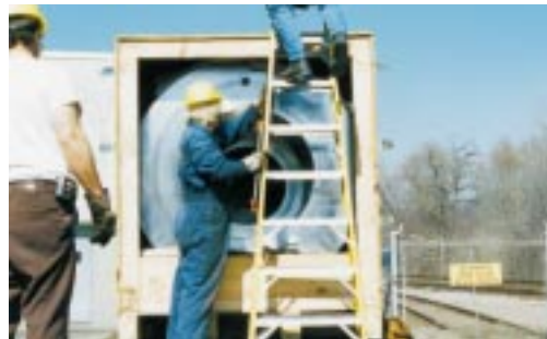
Figure 7-7: Alternative shipping crate for an isostatic press.
