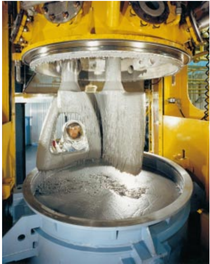
Figure 5-6: Open-blade configuration of a batch mixer.
