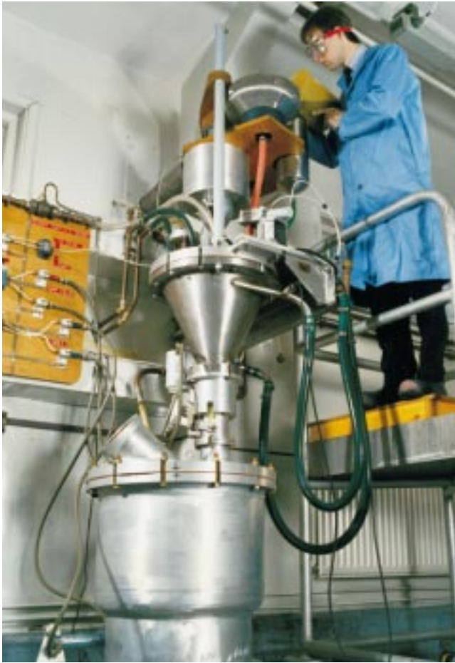
Figure 5-2: Slurry cast double-base mixing equipment for a small motor.
