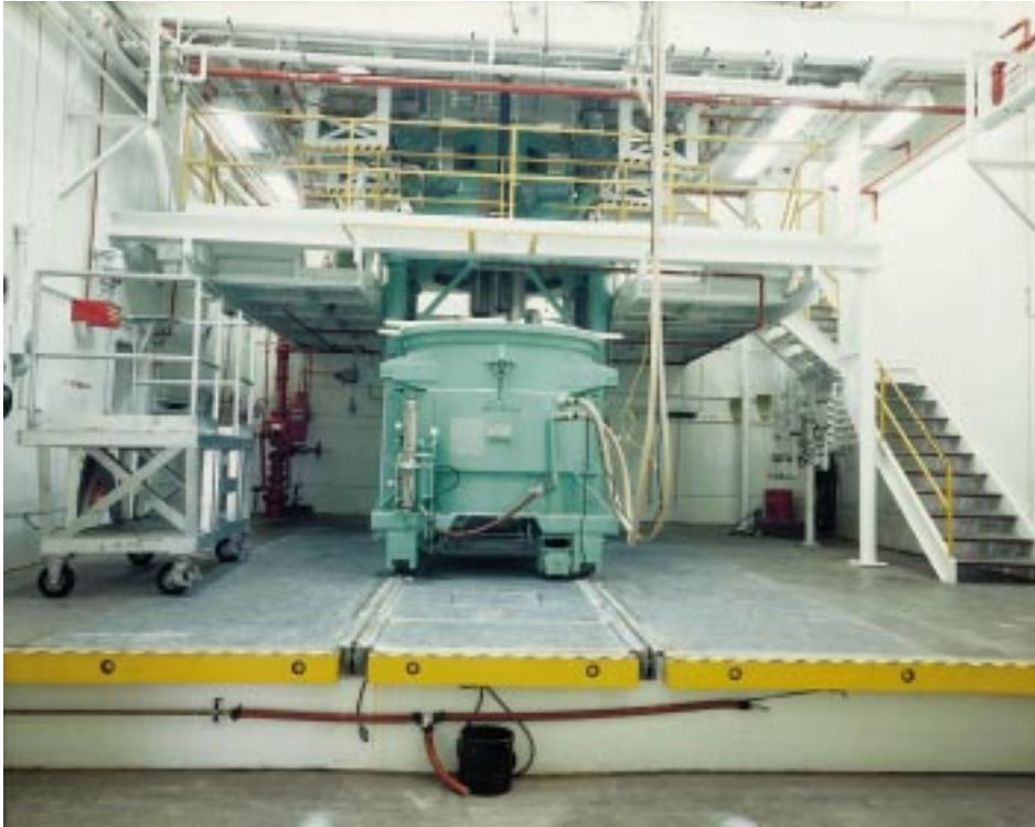
Figure 5-5: A 420-gallon propellant mixing bowl.
