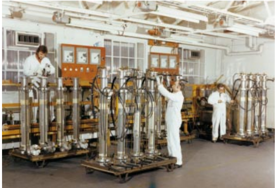
Figure 5-1: Tactical motors with cast-cure tooling attached.
