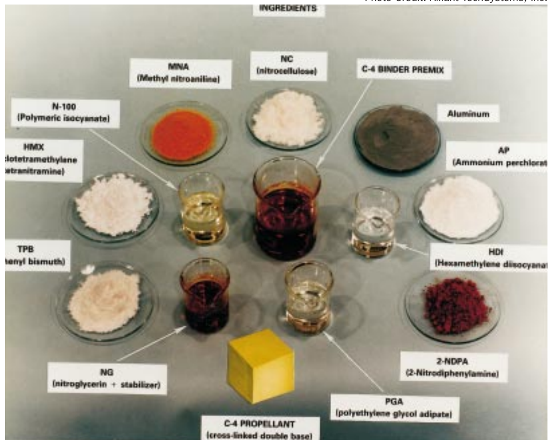
Figure 4-2: Composite-modified double-base propellant and samples of its constituent chemicals.
