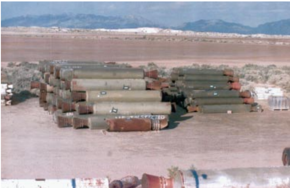
Figure 20-1: On the right, solid rocket motors controlled under Category II. Motors on the left are large enough to be controlled under Item 2, Category I.
