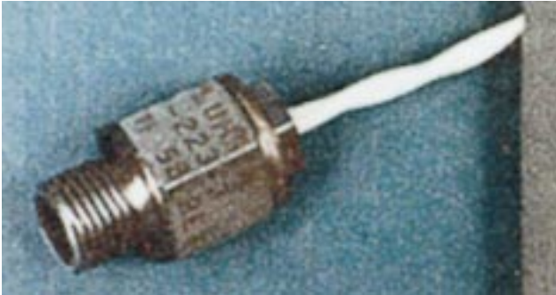
Figure 2-35: A small firing device for an RV that generates a voltage upon impact.
