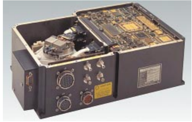
Figure 2-24: A guidance set using hemispheric resonating gyros.
