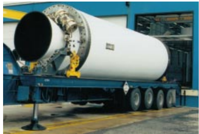
Figure 2-1: A completed stage for a solid propellant missile.
