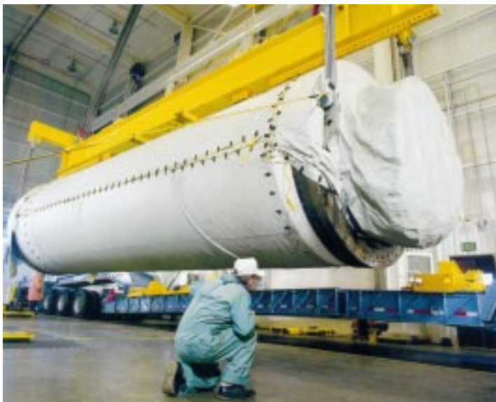
Figure 2-3: A large solid rocket stage being lifted onto its trailer for shipment.
