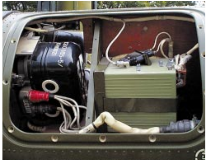
Figure 2-21: An older technology guidance set, comprised of several components, installed in a missile.
