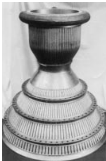
Figure 2-18: Combustion chamber and nozzle throat of a liquid propellant engine.
