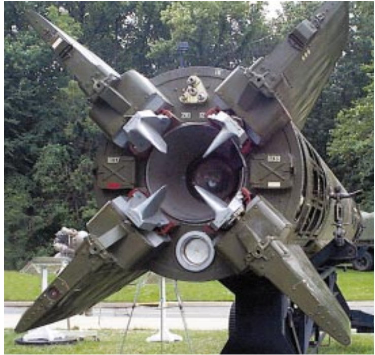
Figure 2-32: Four jet vanes mounted in the aft end of a ballistic missile.
