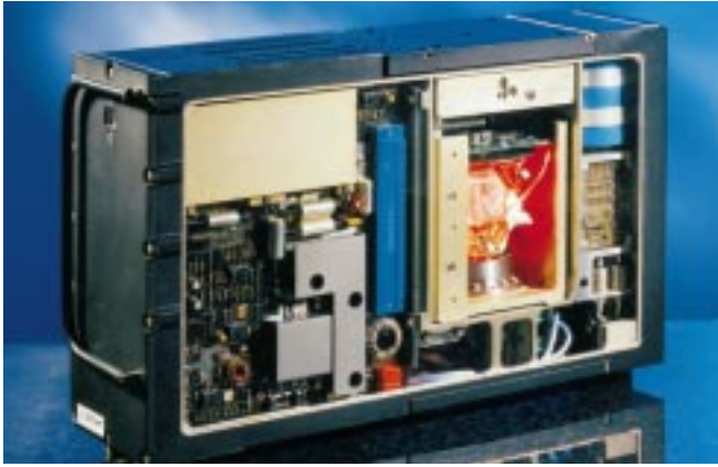
Figure 2-23: A guidance set using ring laser gyros.
