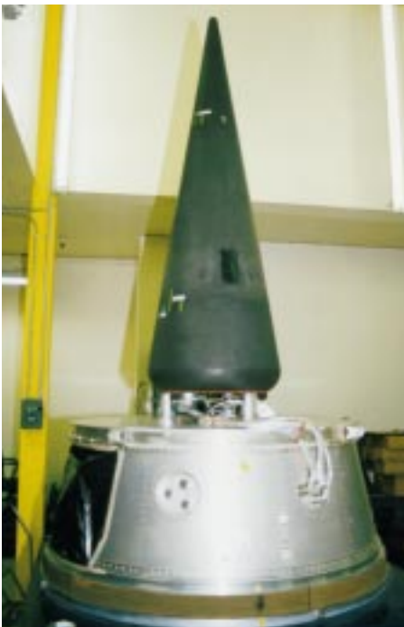
Figure 2-7: A modern RV on its payload support bulkhead.
