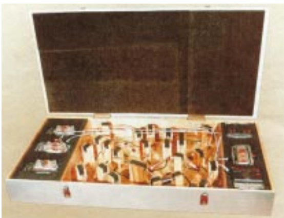
Figure 2-14: An RV radar antenna set packaged for shipment.
