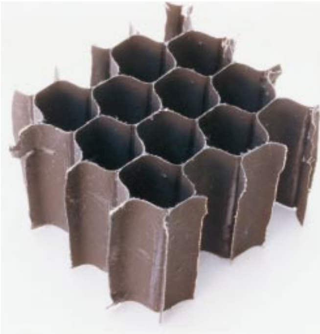
Figure 17-4: A sample of radar absorbing honeycomb material.
