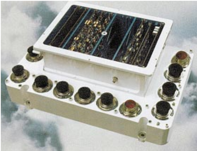
Figure 13-3: A radiation-hardened digital signal processor.
