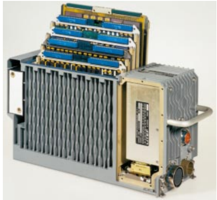
Figure 13-2: A ruggedized computer for fighters, which is similar to a missile or an UAV computer.
