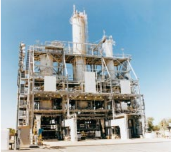
Figure 15-14: A liquid rocket engine test stand with three testing bays. The bay on the right is for testing turbopumps.
