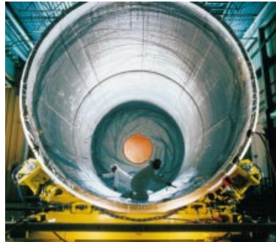
Figure 3-18: Installation of lining inside a motor case.
