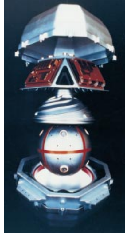
Figure 9-16: A strapdown IMU that contains three accelerometers and three ring laser gyros (in the end opposite the cables).
