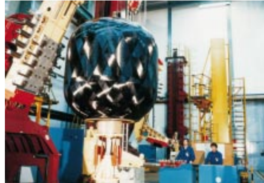
Figure 3-17: A large filament-wound solid rocket motor case.
