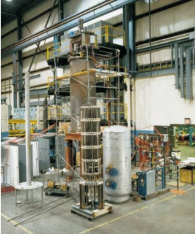
Figure 7-5: An isostatic press in the background, surrounded by a light, metal frame.
