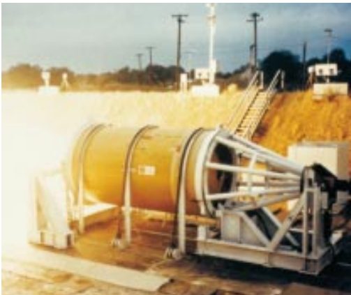
Figure 15-12: An outdoor, horizontal solid rocket motor test stand showing the dolly and frame holding the motor
