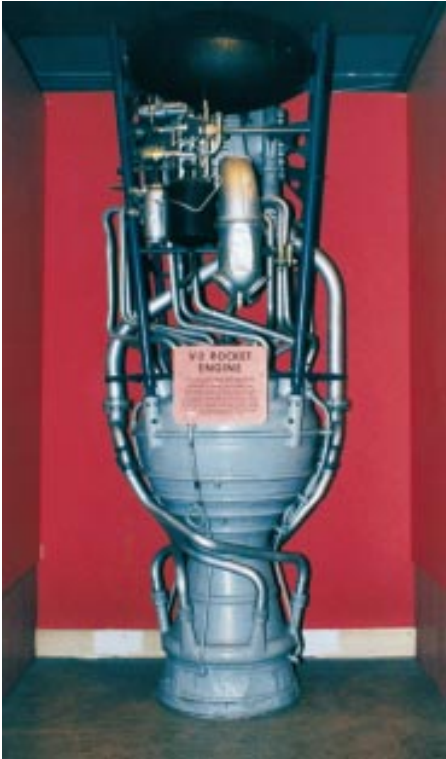
Figure 2-20: A World War II vintage V-2 liquid rocket engine.
