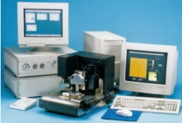
Figure 9-18: A profilometer system used for measuring mirrors.
