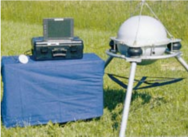
Figure 12-14: A gravity meter that operates suspended from a helicopter. Its associated electronics, shown on the left, are installed in the helicopter.
