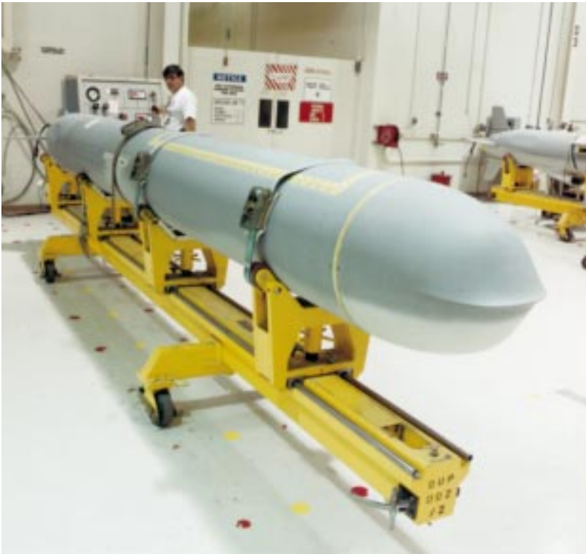
Figure 1-9: An operational cruise missile on its checkout stand showing its nose cone modified to lower radar returns and enhance aerodynamic performance.
