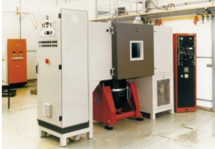
Figure 15-22: A controlled environmental chamber with vibration capability.
