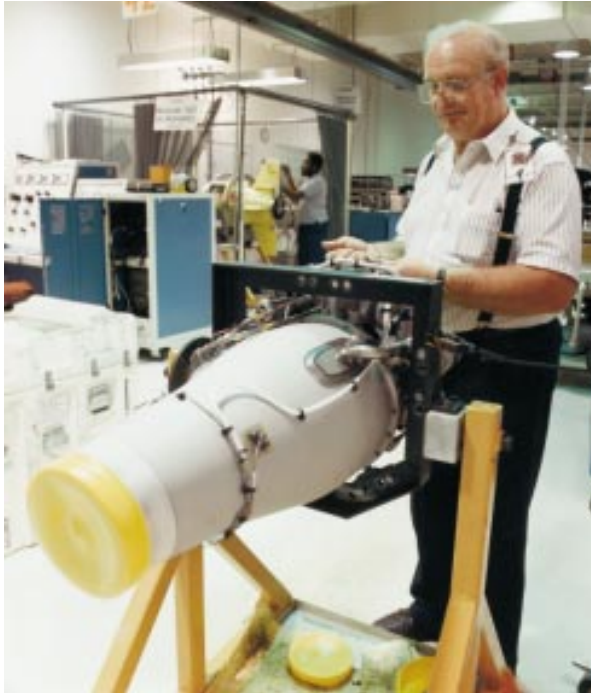
Figure 3-1: A small turbojet engine for a cruise missile on its checkout stand.
