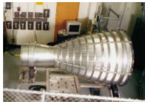
Figure 3-25: Side view of a regeneratively cooled nozzle.
