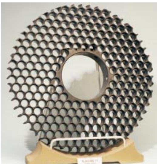
Figure 3-12: A complete ramjet flow straightening device before placement into the inlet duct.
