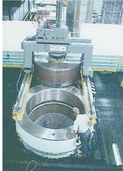
Figure 7-3: A very large isostatic pressure vessel and threaded plug.
