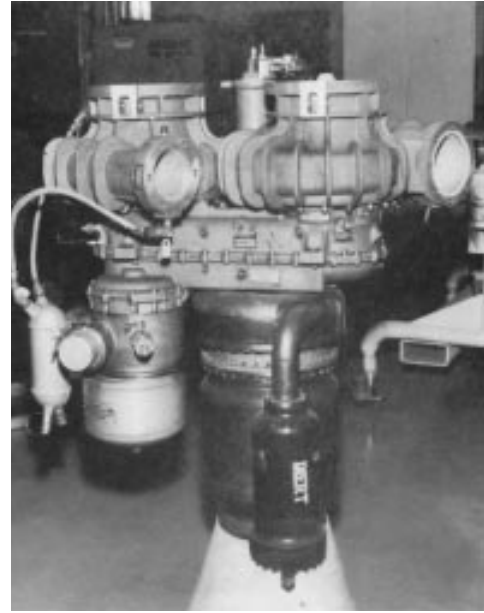
Figure 3-36: A multi-shaft turbopump assembly.
