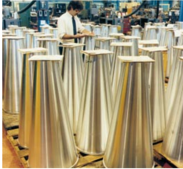
Figure 2-9: Modern RV mid-sections during manufacture.
