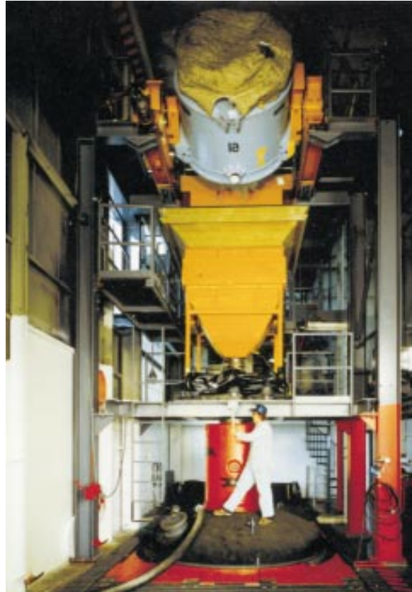
Figure 5-3: A propellant casting pit, with a motor case belowground.
