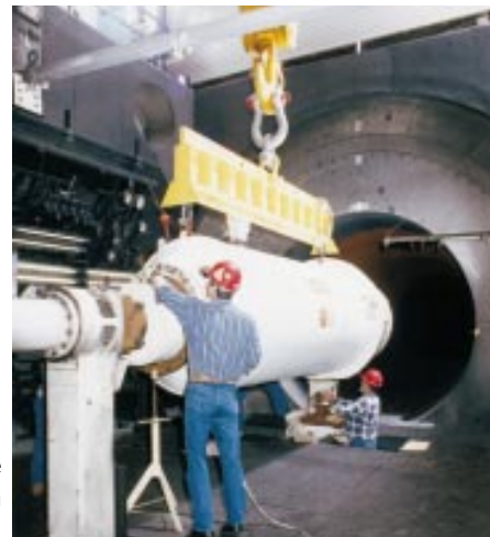
Figure 15-19: A large rocket test facility capable of simulated altitudes of up to 33,000 m.
