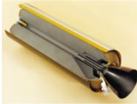
Figure 3-22: A cut-away view of a solid motor that shows how the nozzle fits into the aft end of the motor.
