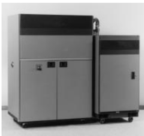
Figure 15-27: A linac RF amplifier on the left with the water pump cabinet on the right.
