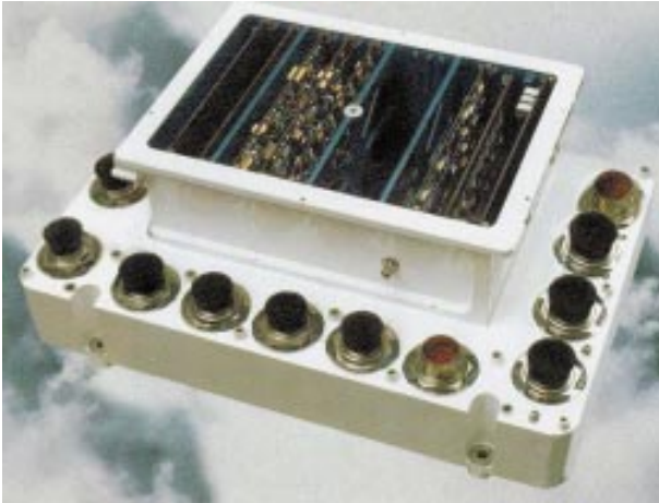
Figure 11-5: Digital signal processor with the lid removed. The size is 5 to 7.5 cm on each side.
