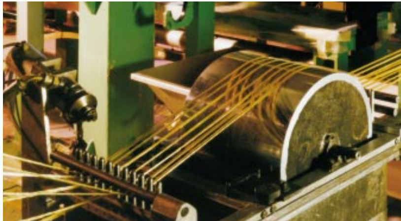
Figure 6-8: A machine adding resin to seven lines of roving.
