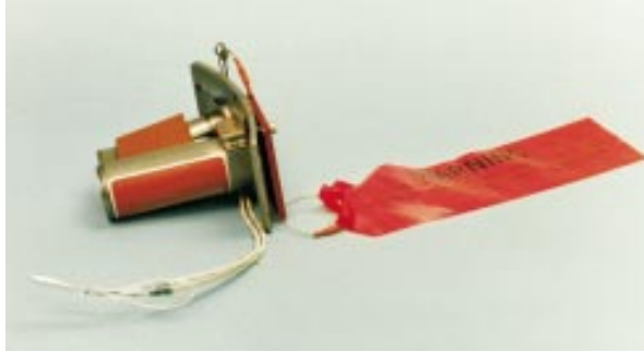
Figure 2-33: A missile fuse with safety plate and warning label.
