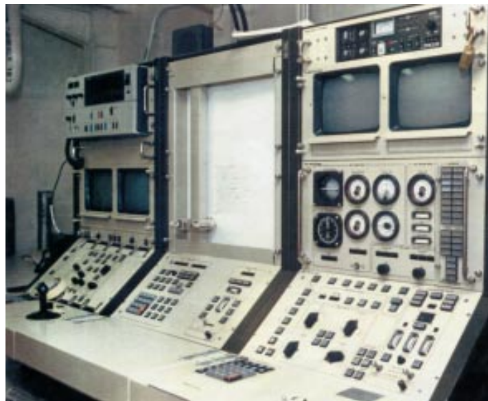
Figure 12-26: An integrated unmanned air vehicle control station.
