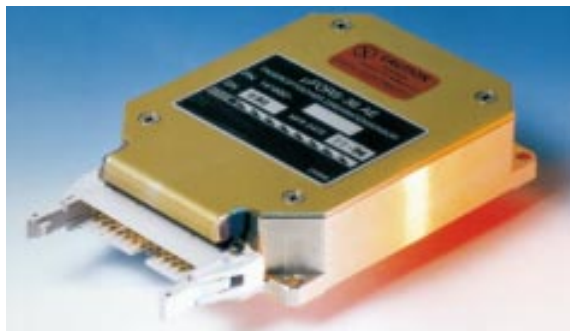
Figure 9-11: A fiber optic, rate sensing gyro. It is 2 × 6.5 × 8 cm.
