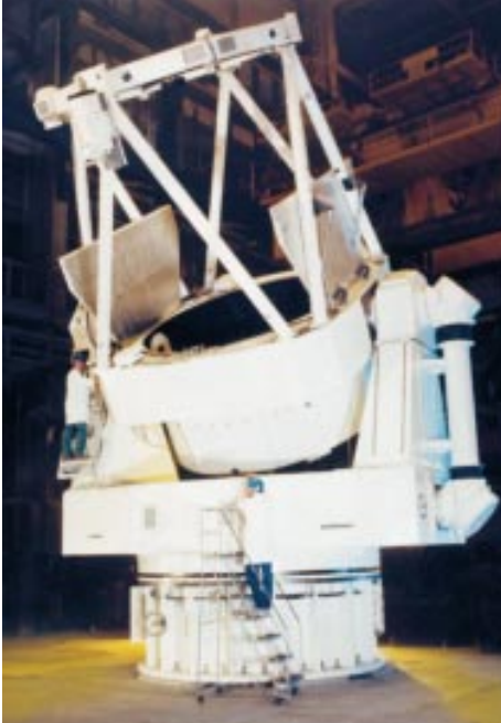
Figure 12-28: An optical missile tracking telescope.
