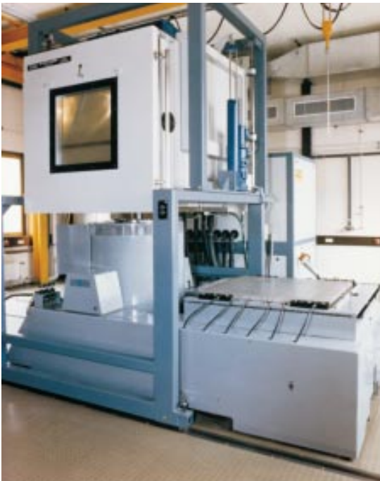
Figure 15-23: Another vibration and environmental test apparatus configuration.
