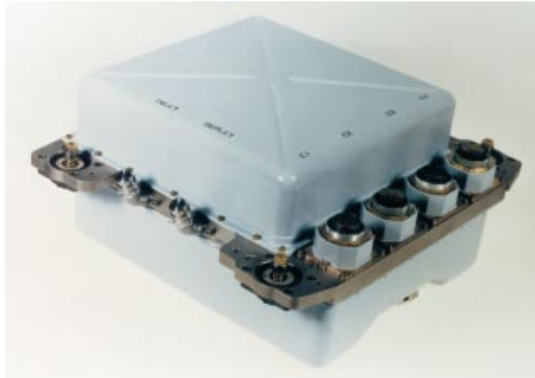
Figure 13-4: A radiation-hardened electronics assembly with liquid cooling.
