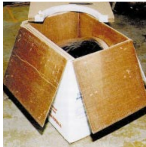
Figure 8-5: View of the prepreg shipping container with the lid open and the support yoke removed.
