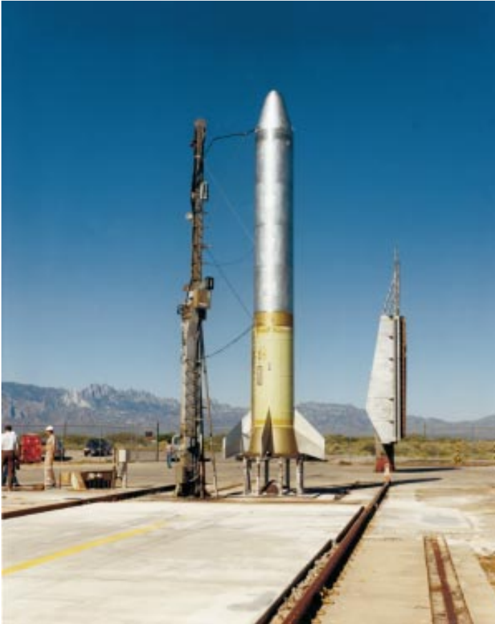
Figure 12-1: Minimal launch pad with a gantry and connections to a complete rocket system.
