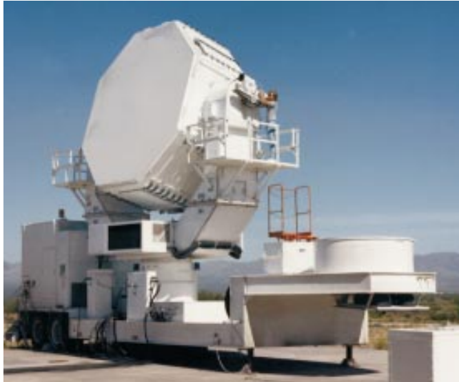
Figure 12-27: A mobile phased array missile tracking radar.
